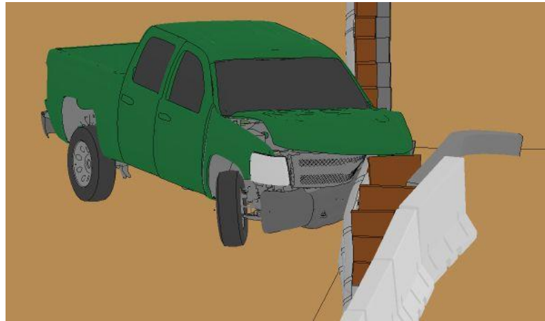
Figure 66. Vehicle Snag on Blockout for Impact Location No. 6 at 90 ms
